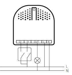
The product must be wired according to the diagram above.
